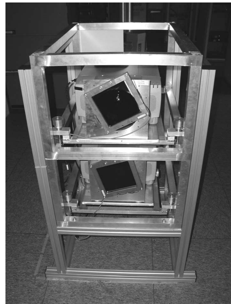
Figure 4. Stereo projection rack with LC-shutters
