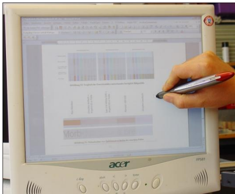
Figure 6: The Anoto pattern enabled 15" Digisketch prototype
