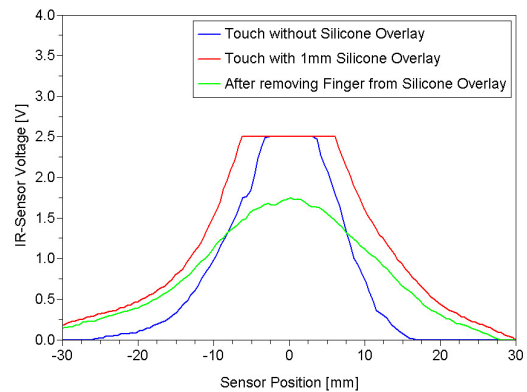
Figure 8: Hysteresis effect of a silicone overlay on a 6 mm acrylic: Because silicone adheres quite well on the FTIR acrylic it sticks to it for a short time (around 3 s) after being touched.
