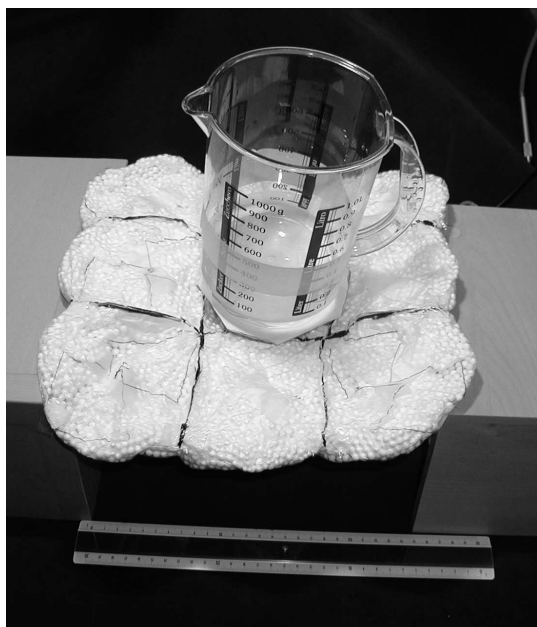
Figure 6: The 3x3 mesh fully extended, carrying 450g
